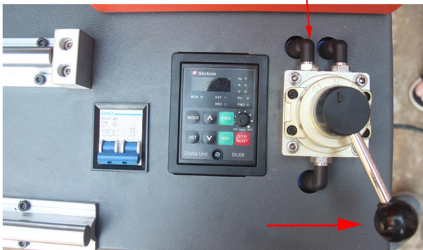
7. Open air valve, pinch roller raised up and fix the belt
