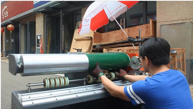
6. Let the belt through the pinch roller
