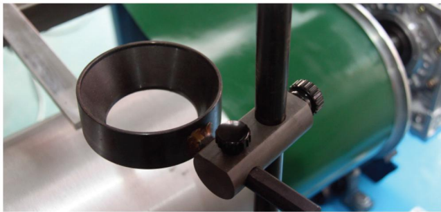
10. Fix the welding gun, adjust the welding position.
