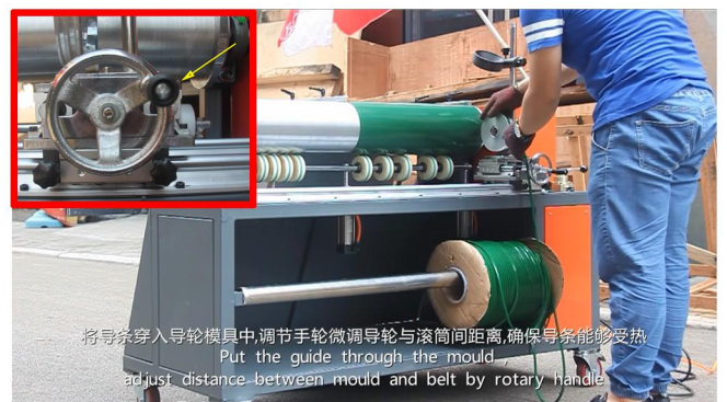
9. Put the guide through the mould, adjust distance between mould the belt by rotary handle.
