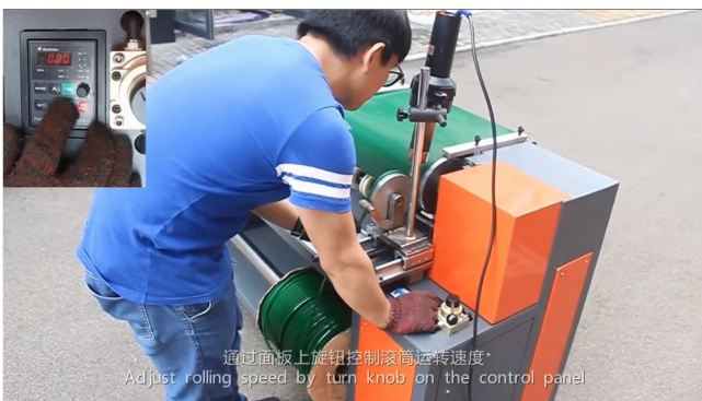
12.Use the speed conroller to welding the V guide
