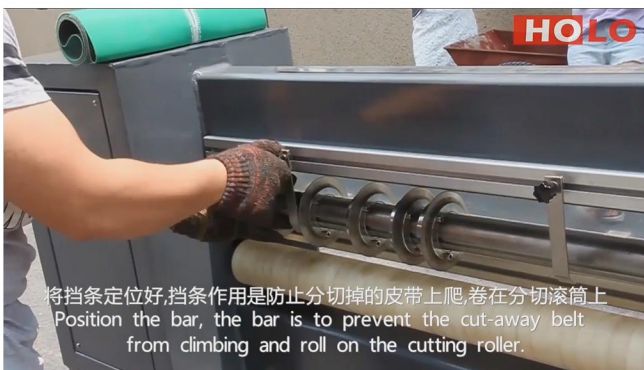
2.Position the bar to prevent the cut-away belt from climbing and roll on the cutting roller
