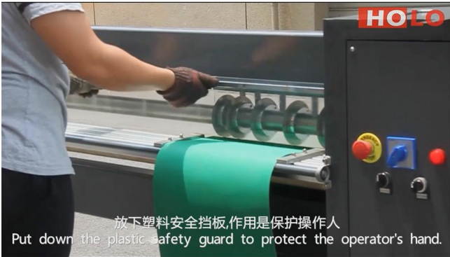
6. Put down the plastic safety Guard to Protect the operator
