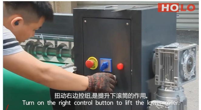
7. Turn on the bottom roll control to raised up the bottom roller
