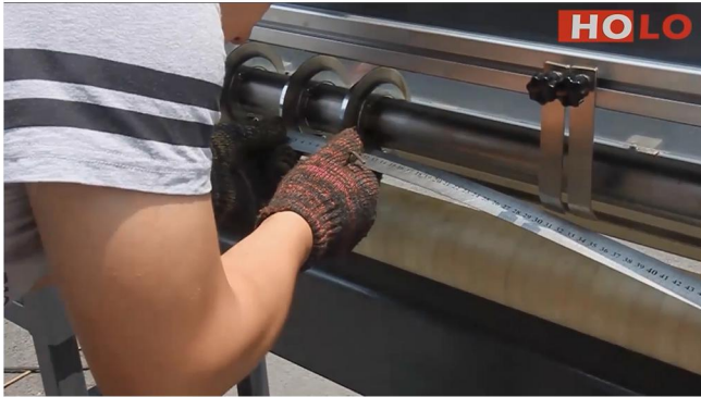
1.Measure the blade distance according to request belt width and fix the round blade
