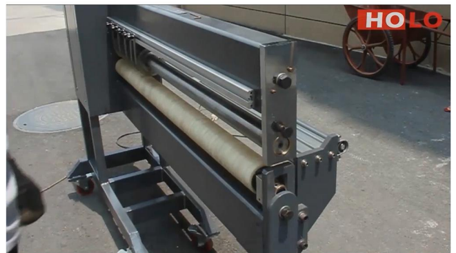
3.Lower the side baffle which is to prevent the machine from being damaged during shipping.
