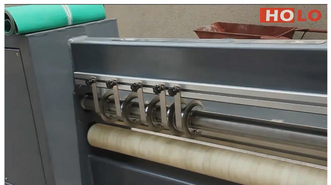
2.Position the bar to prevent the cut-away belt from climbing and roll on the cutting roller
