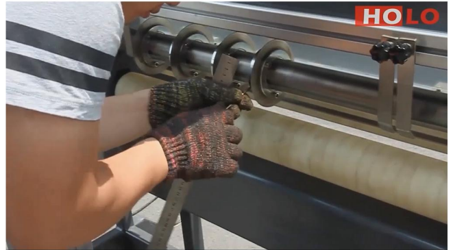
1.Measure the blade distance according to request belt width and fix the round blade
