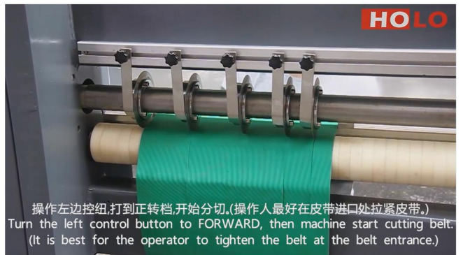
8. Turn the left control to "FORWARD" to cut.
