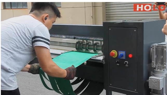
9. Operator better to hold the belt during cutting.
