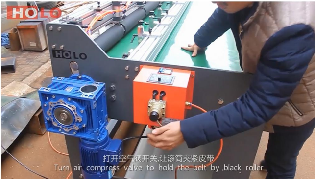
5. Open the air valve to hold the belt by rubber roller
