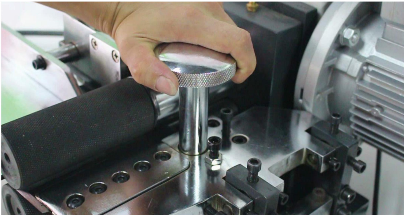
a. Forced rotation the Knife adjusting nut to adjust the height of the knife
