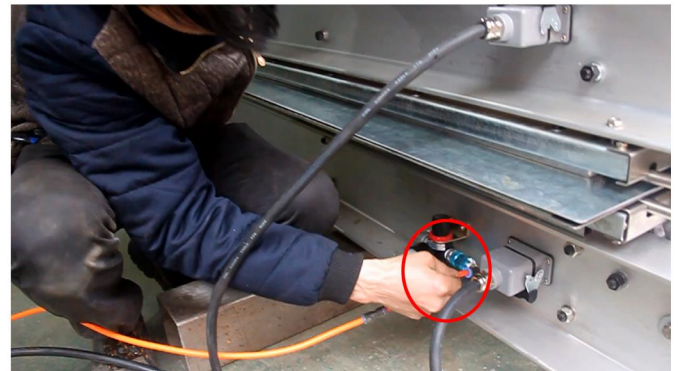
4.Connect Pressure pipe
