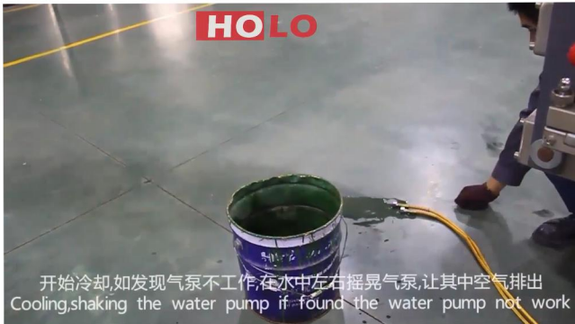
17.If water Pump not work,shake the pump ,get the air outside the pump.
