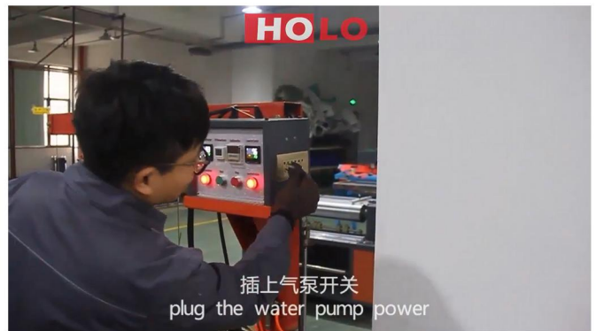
14.Plug the water pump power
