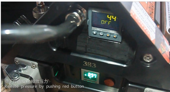
19.Joint work finished ,release pressure (Red Button)
