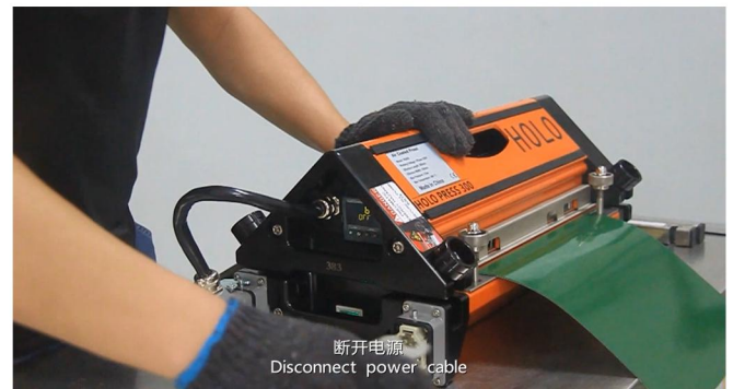
20.Disconnect power cable
