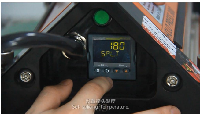
13. Set Splicing Temperature (SPL.T)
